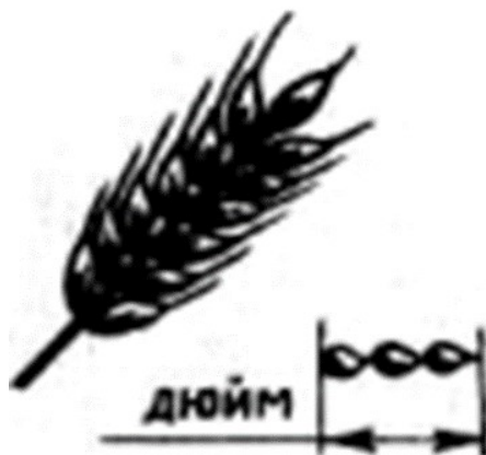
Figure 5. Drawing illustrating the size of the legalized inch.
